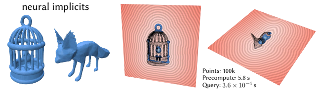
Figure 26. General implicit functions can be turned into signed distance functions by applying our method to a sampling of their zero level set. Here we use the method of Sharp and Jacobson [2022] to sample neural implicits by casting rays. Query times are measured without GPU acceleration.
