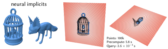
Fig. 5.10: General implicit functions can be turned into signed distance functions by applying our method to a sampling of their zero level set. Here we use the method of Sharp and Jacobson [2022] to sample neural implicits by casting rays. Query times are measured without GPU acceleration.
